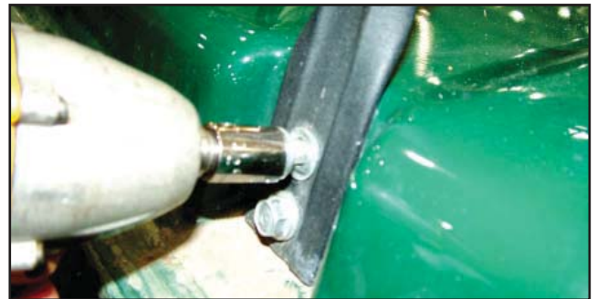
Fig. 2 - Remove Seat Back Support
