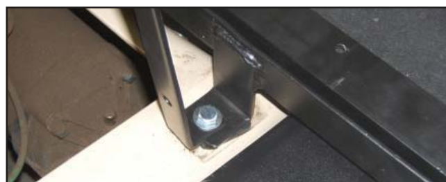
Fig. 8 - Seat Back Support onto Deck Mount Tab
