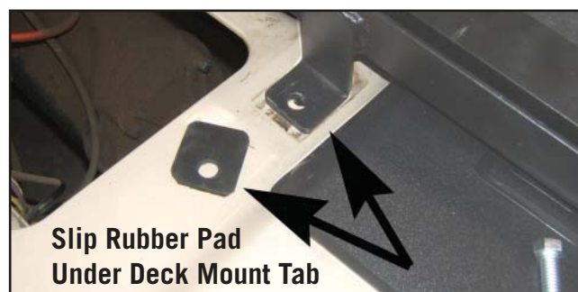
Fig. 7 - Rubber Pad Installation
