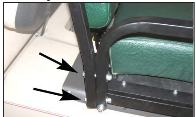
Fig. 14 - Install Top Supports
