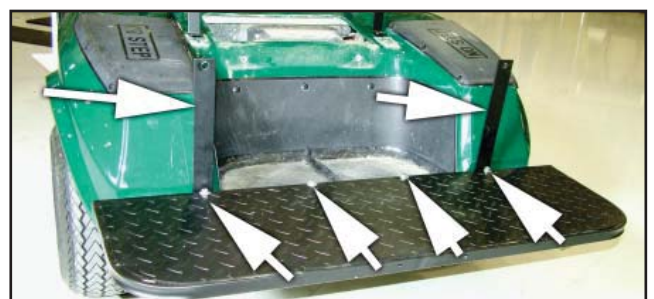
Fig. 4 - Install Rear Foot Rest Assembly
